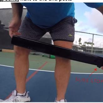
Carefully slide them together until the welded steel stop rests against the end post section.
