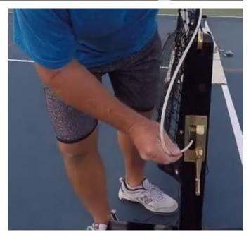
Insert brass handle and screw until tight. Wind the crank until the net is somewhat tight, but don't over tighten.
